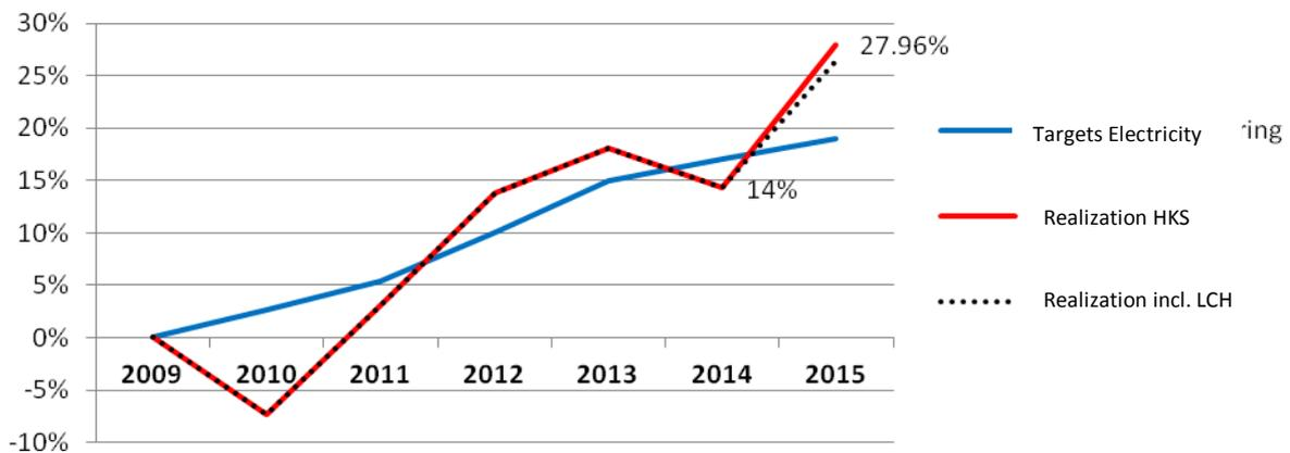
A number of actions intended to reduce electricity consumption by the specified 2% were identified and partly implemented in 2015. These included the more efficient use of lighting and the reduction of compressed air leakage losses.
